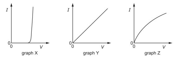
The components are a metal wire at constant temperature, a semiconductor diode and a filament lamp.
