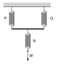
Springs P and Q are identical and each has spring constant *k*. Spring R has spring constant 3*k*.
