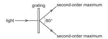
The angle between the second-order diffraction maxima is 80°, as shown.
